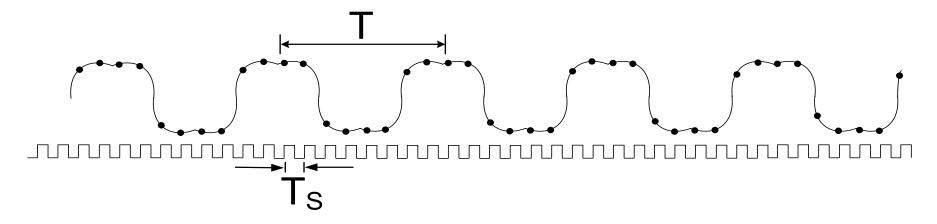
THEOREM (conceptual): If a band-limited periodic signal is sampled at a rate that exceeds the Nyquist rate, then the Fourier Series coefficients can be directly obtained from the DFT of a sampled sequence.
