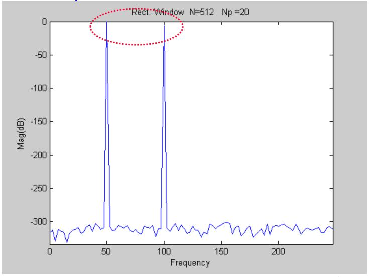
DFT Horizontal Axis Converter to Frequency :  $f_{AXIS} = f_{SIGNAL} \frac{n-1}{N_p}$
