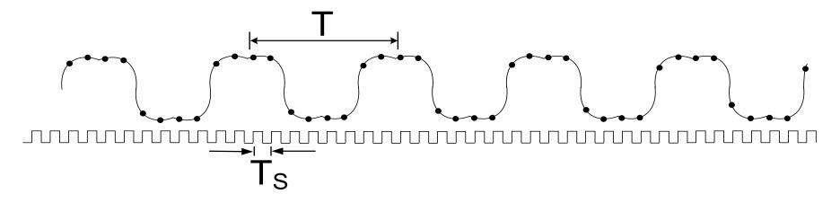
Observation: If a band-limited periodic signal is sampled over an integral number of periods at a rate that exceeds the Nyquist rate, then the Fourier Series coefficients can be directly obtained from the sampled sequence.
