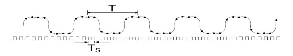
Consider sampling x(t) at uniformly spaced points in time  $T_{\text{S}}$  seconds apart
