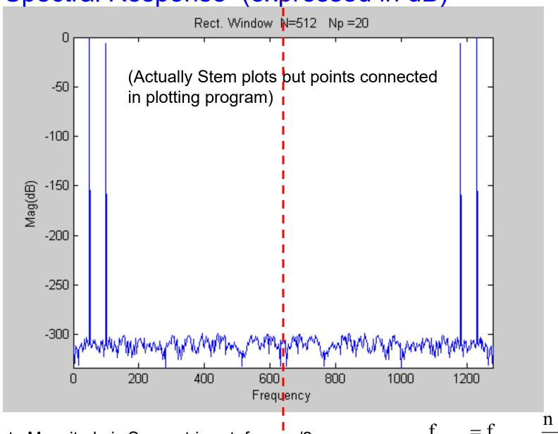
Note Magnitude is Symmetric wrt  $f_{SAMPLE}/2$   $f_{AXIS} = f_{SIGNAL}/2$
